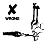
WILL WORK CORRECTLY ON AUTOMATIC RELEASE BUT THE LIFERAFT WILL ONLY BE SECURED BY THE WEAK LINK IF THROWN OVERBOARD - WEAK LINK MAY BREAK AND LIFERAFT WILL BE LOST
