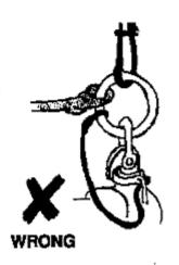
LIFERAFT WILL NOT RELEASE FROM CRADLE IF THE SHIP SINKS LIFERAFT WILL NOT RELEASE FROM CRADLE IF THE SHIP SINKS
