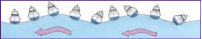
A change of heading and/or speed reduces resonant rolling motions.
